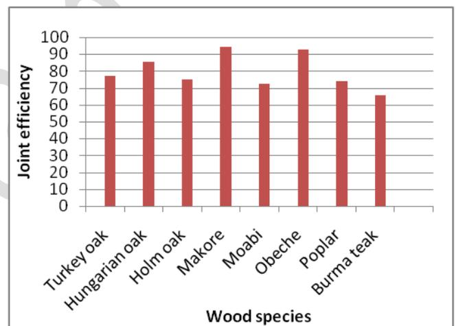
Fig. 2 Comparison of finger joint efficiencies of different wood species with types of wood species
