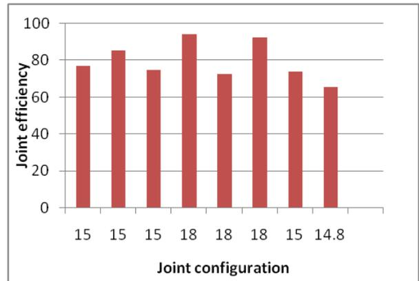
Fig. 1 Comparison of finger joint efficiencies of different wood species for different joint configurations
