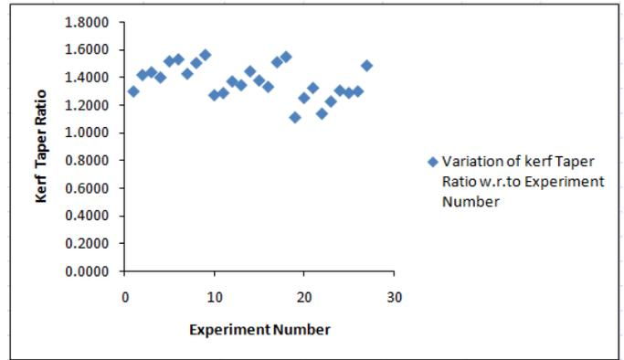
Figure 2: Variation of Kerf Taper Ratio with respect to Experiment Number
