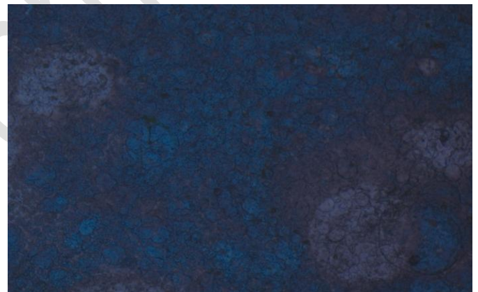
Fig5. OM image of RIVPSE based PS sample HF:HNO 3 (6:1) showing islands
