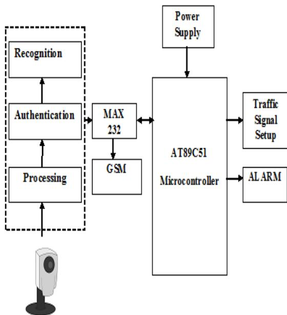
Fig 2 – Block Diagram of ALPR System
