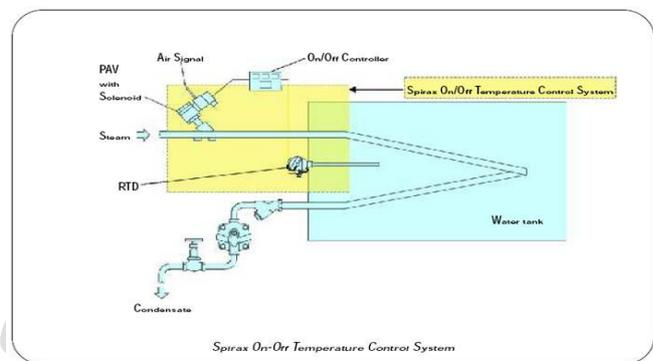
Fig .9.on-off temperature control system
