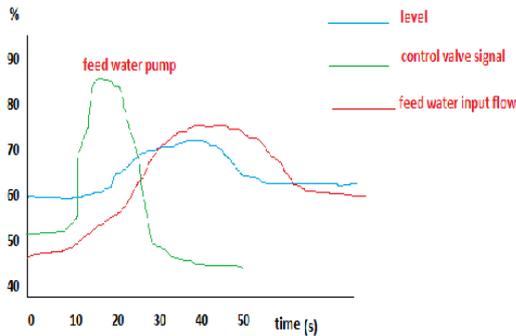
Fig 8.two element control
