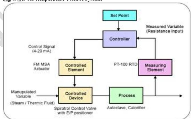
Fig .10.PID temperature control system
