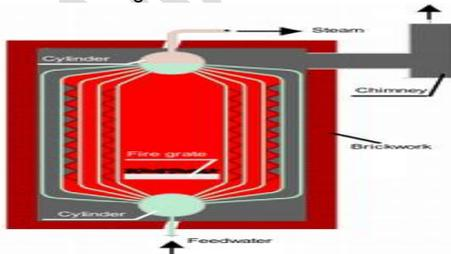
Fig.2.Water tube boiler
