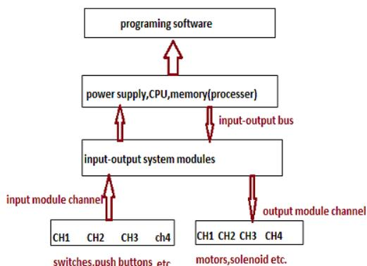
fig.11.PLC block diagram
